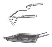
The handle makes it easier to take the universal tray, baking tray and rack out of the oven, or to put them into it. The two prongs at the top go inside the tray or above the rack and the U-shaped supports underneath.
